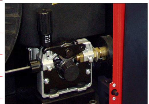
Foto del vano bobina con trainafilo a 2 rulli Photo of the spool compartment with 2-roller wire feeder.
