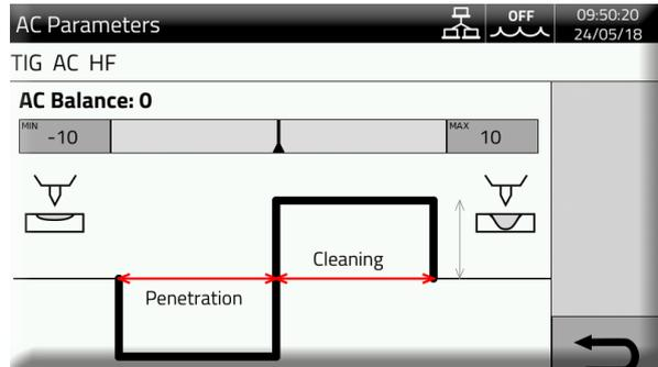
**WIN TIG AC-DC 450 T ( art.396 )** is a three-phase power source with inverter technology for TIG (pulsed) and electrode (MMA) AC DC welding, with built-in HF ignition. Supplied with cooling unit and also with trolley for transportation of the power source.
