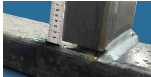
Mild steel / fillet Thickness 2mm, current 110A Unified voltage Clearance 3mm, welding speed 50cm/min
