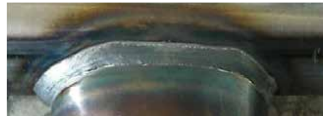
Mild steel / intersecting wire welding Thickness 1.5mm, Current 95A, Voltage 17V Welding speed 50cm/min Gas (20% Ar + 80% CO 2 )
